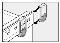
■ Slide the markers onto the guide runners on the edge of the drawers.
